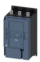
SIRIUS soft starter 200-480 V 315 A, 24 V AC/DC Screw terminals Thermistor input
