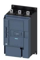
SIRIUS soft starter 200-600 V 210 A, 24 V AC/DC spring-type terminals Thermistor input
