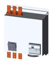
SIRIUS soft starter Values at 575 V, 50 °C standard: 970 A, 1100 hp Inside-delta: 1680 A, 1900 hp 400-690 V AC, 115 V AC Screw terminals !!! Phased-out product !!! Successor is SIRIUS 3RW5, Preferred successor type is >>3RW5558-6HA16<<
