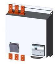
SIRIUS soft starter Values at 460 V, 50 °C standard: 970 A, 850 hp Inside-delta: 1680 A, 1500 hp 200-460 V AC, 115 V AC spring-type terminals !!! Phased-out product !!! Successor is SIRIUS 3RW5, Preferred successor type is >>3RW5558-2HA14<<
