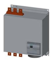
SIRIUS soft starter Values at 500 V, 40 °C standard: 880 A, 630 kW Inside-delta: 1524 A, 1000 kW 400-600 V AC, 230 V AC Screw terminals !!! Phased-out product !!! Successor is SIRIUS 3RW5, Preferred successor type is >>3RW5556-6HA16<<
