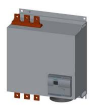
SIRIUS soft starter Values at 500 V, 40 °C standard: 880 A, 630 kW Inside-delta: 1524 A, 1000 kW 400-600 V AC, 230 V AC spring-type terminals !!! Phased-out product !!! Successor is SIRIUS 3RW5, Preferred successor type is >>3RW5556-2HA16<<
