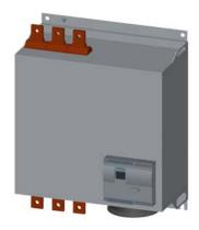
SIRIUS soft starter Values at 575 V, 50 °C standard: 780 A, 850 hp Inside-delta: 1351 A, 1500 hp 400-690 V AC, 115 V AC spring-type terminals !!! Phased-out product !!! Successor is SIRIUS 3RW5, Preferred successor type is >>3RW5556-2HA16<<
