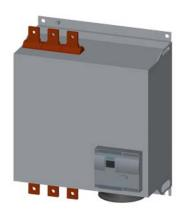
SIRIUS soft starter Values at 460 V, 50 °C standard: 780 A, 700 hp Inside-delta: 1351 A, 1200 hp 200-460 V AC, 115 V AC spring-type terminals !!! Phased-out product !!! Successor is SIRIUS 3RW5, Preferred successor type is >>3RW5556-2HA14<<
