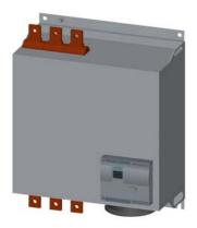
SIRIUS soft starter Values at 575 V, 50 °C standard: 693 A, 750 hp Inside-delta: 1200 A, 1350 hp 400-600 V AC, 115 V AC spring-type terminals !!! Phased-out product !!! Successor is SIRIUS 3RW5, Preferred successor type is >>3RW5554-2HA16<<
