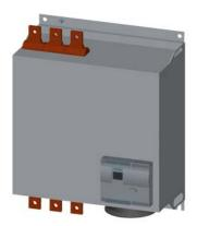
SIRIUS soft starter Values at 400 V, 40 °C standard: 693 A, 400 kW Inside-delta: 1200 A, 710 kW 200-460 V AC, 230 V AC spring-type terminals !!! Phased-out product !!! Successor is SIRIUS 3RW5, Preferred successor type is >>3RW5553-2HA14<<
