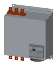
SIRIUS soft starter Values at 460 V, 50 °C standard: 551 A, 450 hp Inside-delta: 954 A, 850 hp 200-460 V AC, 115 V AC Screw terminals !!! Phased-out product !!! Successor is SIRIUS 3RW5, Preferred successor type is >>3RW5552-6HA14<<
