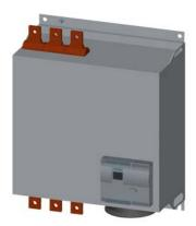
SIRIUS soft starter Values at 400 V, 40 °C standard: 615 A, 355 kW Inside-delta: 1065 A, 630 kW 200-460 V AC, 230 V AC spring-type terminals !!! Phased-out product !!! Successor is SIRIUS 3RW5, Preferred successor type is >>3RW5552-2HA14<<
