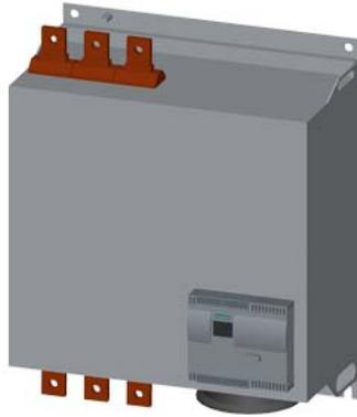
SIRIUS soft starter Values at 575 V, 50 °C standard: 494 A, 500 hp Inside-delta: 856 A, 950 hp 400-690 V AC, 115 V AC spring-type terminals !!! Phased-out product !!! Successor is SIRIUS 3RW5, Preferred successor type is >>3RW5548-2HA16<<
