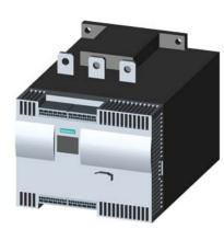
SIRIUS soft starter Values at 690 V, 40 °C standard: 432 A, 400 kW Inside-delta: only up to 600 V 400-690 V AC, 230 V AC spring-type terminals !!! Phased-out product !!! Successor is SIRIUS 3RW5, Preferred successor type is >>3RW5547-2HA16<<
