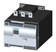
SIRIUS soft starter Values at 575 V, 50 °C standard: 280 A, 250 hp Inside-delta: 485 A, 500 hp 400-690 V AC, 115 V AC spring-type terminals !!! Phased-out product !!! Successor is SIRIUS 3RW5, Preferred successor type is >>3RW5545-2HA16<<
