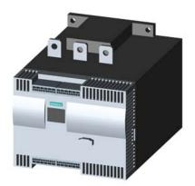
SIRIUS soft starter Values at 575 V, 50 °C standard: 215 A, 200 hp Inside-delta: 372 A, 350 hp 400-600 V AC, 115 V AC spring-type terminals !!! Phased-out product !!! Successor is SIRIUS 3RW5, Preferred successor type is >>3RW5544-2HA16<<
