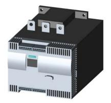
SIRIUS soft starter Values at 400 V, 40 °C standard: 203 A, 110 kW Inside-delta: 352 A, 200 kW 200-460 V AC, 230 V AC spring-type terminals !!! Phased-out product !!! Successor is SIRIUS 3RW5, Preferred successor type is >>3RW5543-2HA14<<
