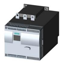
SIRIUS soft starter Values at 400 V, 40 °C standard: 162 A, 90 kW Inside-delta: 281 A, 160 kW 200-460 V AC, 230 V AC spring-type terminals !!! Phased-out product !!! Successor is SIRIUS 3RW5, Preferred successor type is >>3RW5536-2HA14<<
