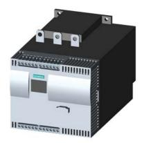
SIRIUS soft starter Values at 400 V, 40 °C standard: 113 A, 55 kW Inside-delta: 196 A, 110 kW 200-460 V AC, 230 V AC spring-type terminals !!! Phased-out product !!! Successor is SIRIUS 3RW5, Preferred successor type is >>3RW5534-2HA14<<
