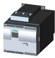
SIRIUS soft starter Values at 460 V, 50 °C standard: 82 A, 60 hp Inside-delta: 142 A, 100 hp 200-460 V AC, 115 V AC spring-type terminals !!! Phased-out product !!! Successor is SIRIUS 3RW5, Preferred successor type is >>3RW5527-3HA14<<
