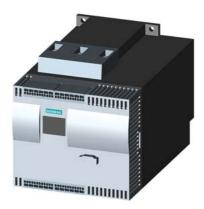
SIRIUS soft starter Values at 500 V, 40 °C standard: 77 A, 45 kW Inside-delta: 133 A, 90 kW 400-600 V AC, 230 V AC spring-type terminals !!! Phased-out product !!! Successor is SIRIUS 3RW5, Preferred successor type is >>3RW5526-3HA16<<
