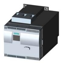
SIRIUS soft starter Values at 575 V, 50 °C standard: 68 A, 50 hp Inside-delta: 118 A, 100 hp 400-690 V AC, 115 V AC spring-type terminals !!! Phased-out product !!! Successor is SIRIUS 3RW5, Preferred successor type is >>3RW5526-3HA16<<
