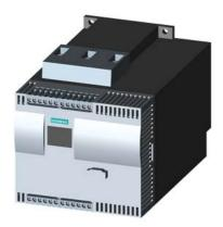
SIRIUS soft starter Values at 575 V, 50 °C standard: 68 A, 50 hp Inside-delta: 118 A, 100 hp 400-690 V AC, 115 V AC Screw terminals !!! Phased-out product !!! Successor is SIRIUS 3RW5, Preferred successor type is >>3RW5526-1HA16<<
