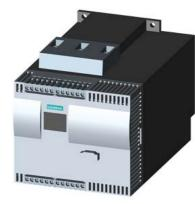
SIRIUS soft starter Values at 460 V, 50 °C standard: 51 A, 30 hp Inside-delta: 88 A, 60 hp 200-460 V AC, 115 V AC Screw terminals !!! Phased-out product !!! Successor is SIRIUS 3RW5, Preferred successor type is >>3RW5525-1HA14<<
