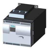
SIRIUS soft starter Values at 460 V, 50 °C standard: 42 A, 25 hp Inside-delta: 73 A, 50 hp 200-460 V AC, 115 V AC spring-type terminals !!! Phased-out product !!! Successor is SIRIUS 3RW5, Preferred successor type is >>3RW5524-3HA14<<
