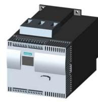
SIRIUS soft starter Values at 575 V, 50 °C standard: 42 A, 30 hp Inside-delta: 73 A, 60 hp 400-600 V AC, 115 V AC Screw terminals !!! Phased-out product !!! Successor is SIRIUS 3RW5, Preferred successor type is >>3RW5524-1HA16<<
