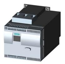
SIRIUS soft starter Values at 575 V, 50 °C standard: 32 A, 25 hp Inside-delta: 55 A, 50 hp 400-600 V AC, 115 V AC Screw terminals !!! Phased-out product !!! Successor is SIRIUS 3RW5, Preferred successor type is >>3RW5517-1HA15<<
