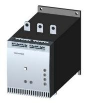
SIRIUS soft starter S6 134 A, 75 kW/400 V, 40 °C 200-460 V AC, 230 V AC spring-type terminals !!! Phased-out product !!! Successor is SIRIUS 3RW5, Preferred successor type is >>3RW5055-2AB14<<
