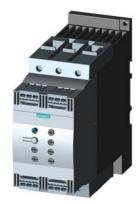
SIRIUS soft starter S3 80 A, 55 kW/500 V, 40  $^\circ\text{C}$  400-600 V AC, 110-230 V AC/DC spring-type terminals
