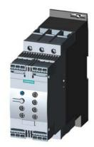
SIRIUS soft starter S2 63 A, 37 kW/500 V, 40  $^{\circ}\text{C}$  400-600 V AC, 24 V AC/DC spring-type terminals Thermistor motor protection
