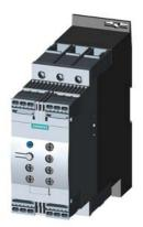
SIRIUS soft starter S2 63 A, 30 kW/400 V, 40 °C 200-480 V AC, 24 V AC/DC spring-type terminals Thermistor motor protection
