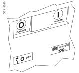
Circuit breaker closed and discharged
