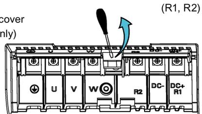
To open the lower cover, pull the locking latch of the cover upwards with a flat-bit screwdriver.
