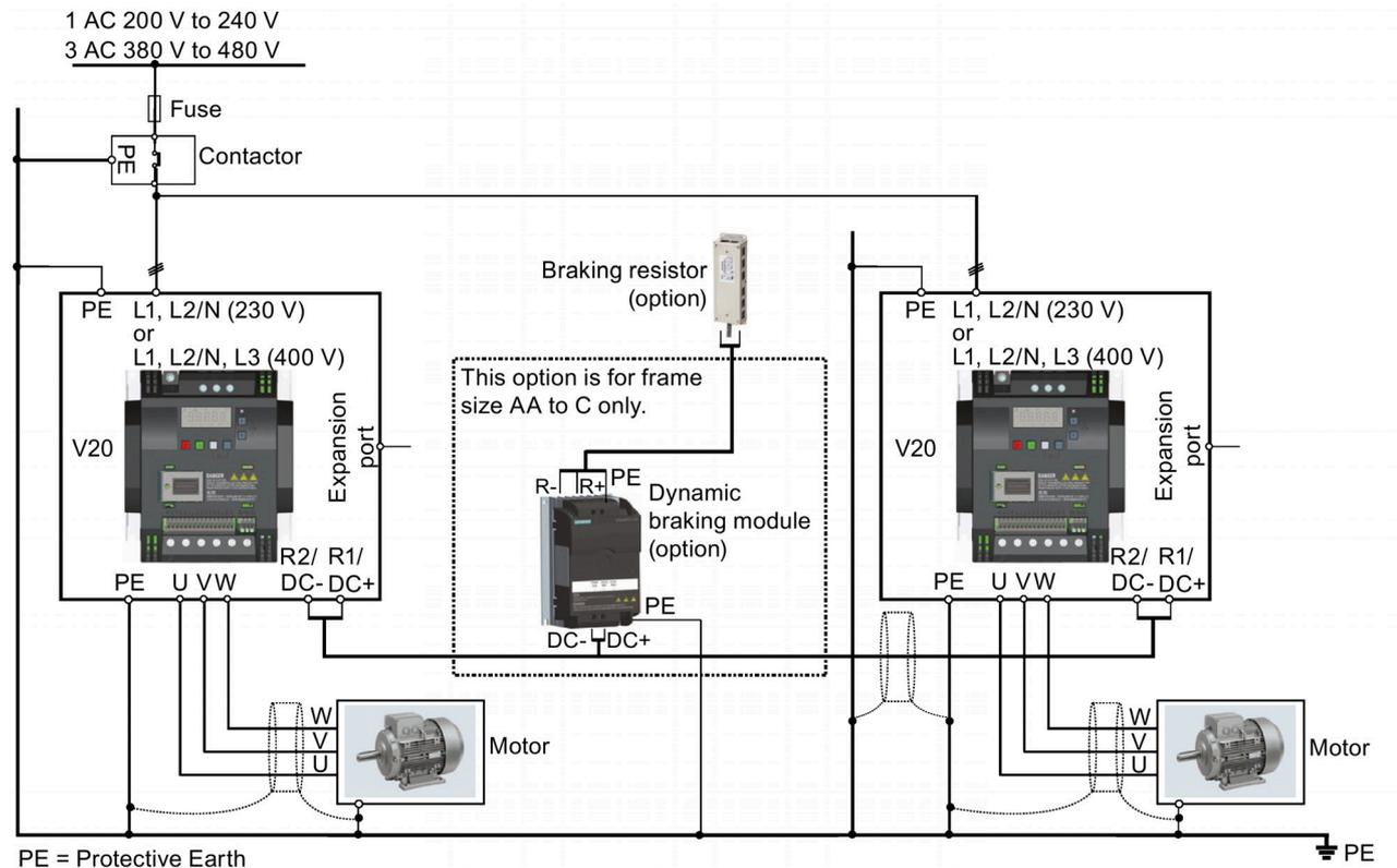
See Section "Terminal description (Page 45)" for the recommended cable cross-sections and screw tightening torques.
