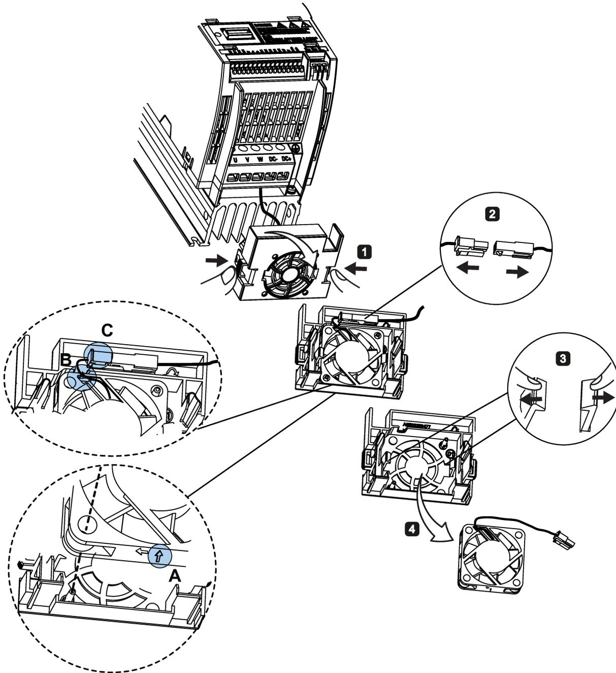
Replacing the fan(s) from FSB, FSC or FSD
