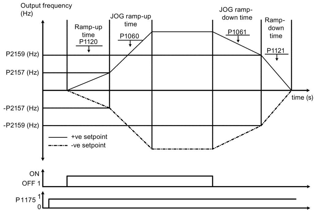
Note that the dual ramp algorithm uses r2198 bits 1 and 2 to determine ( $f_{act} > P2157$ ) and ( $f_{act} < P2159$ ).
