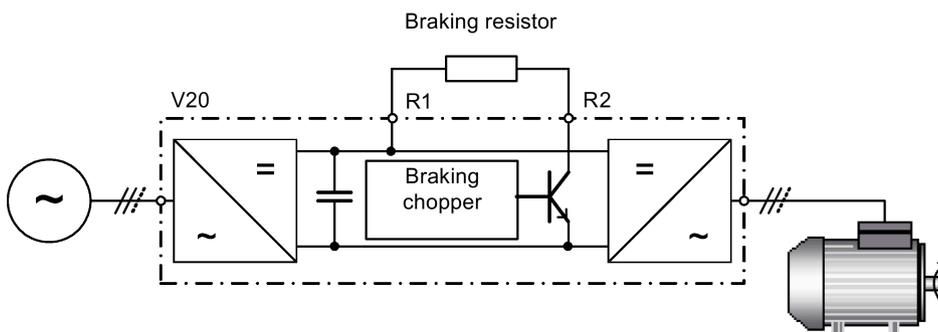
The continuous power  $P_{DB}$  and the duty cycle for the braking resistor can be modified using the dynamic braking module (for frame size AA to C) or parameter P1237 (for frame size D and E).
