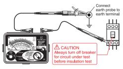
Check the circuit under test is not energized as follows.
