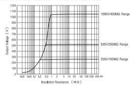
Principle of Insulation Resistance Measurement Resistance value can be obtained by applying a certain high voltage to the resistance (insulation resistance) and measuring the flowing current.
