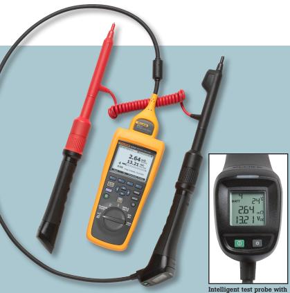
Intelligent test probe wit integrated LCD display
