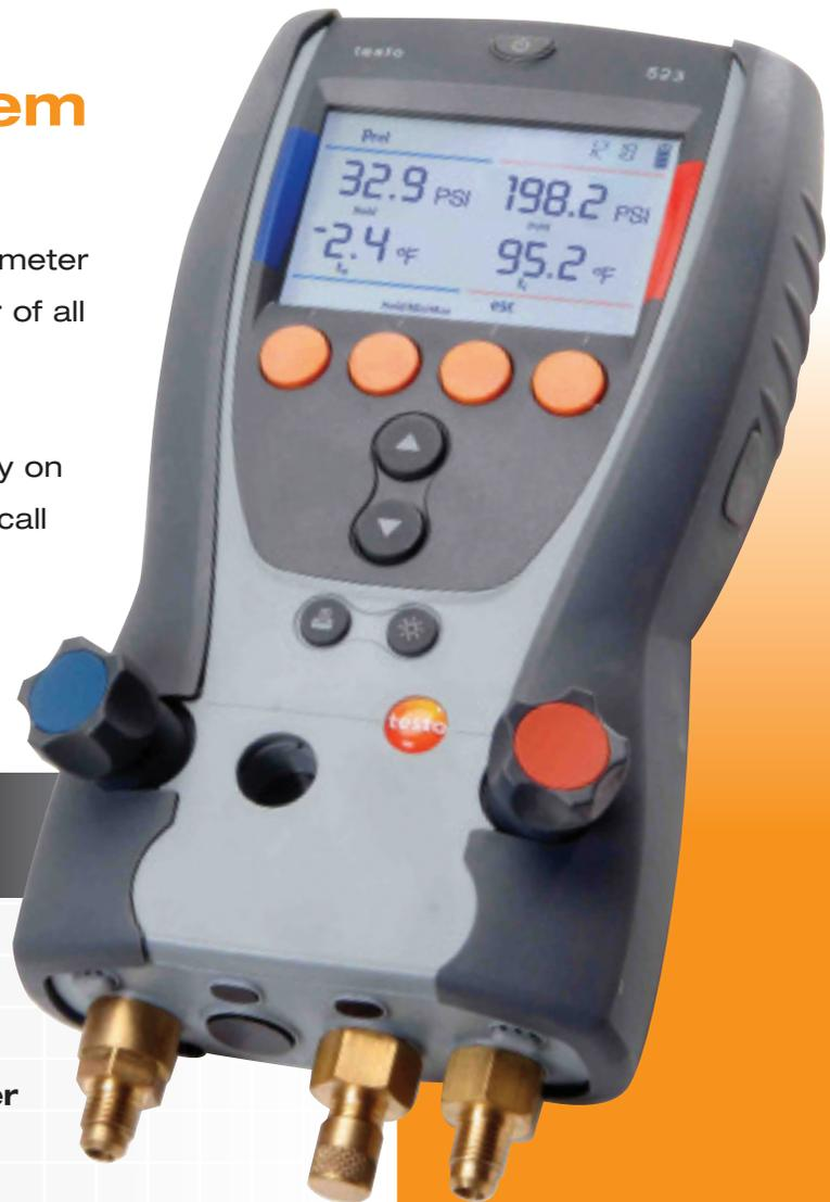
**Real-time superheat and subcooling readings**
