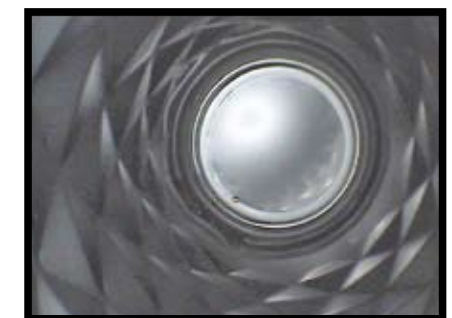
Image with WiDER™ gain applied. WiDER™ gain brightens the darker areas while maintaining the light level and details shown in the bright area.
