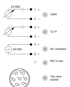
DC: Supply transmitter AC: Supply ventilator
